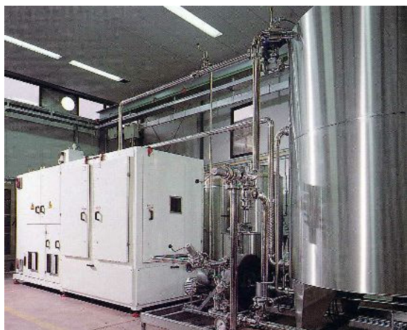
"RF/L 85 kW" equipment for the pasteurisation of fruit preparations for yogurt.
