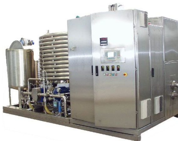
"RF/L 30 kW" equipment for the pasteurisation and sterilisation of viscous liquids.
