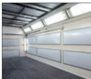
photo 4 Paint drying booth for vehicles and industrial machinery
