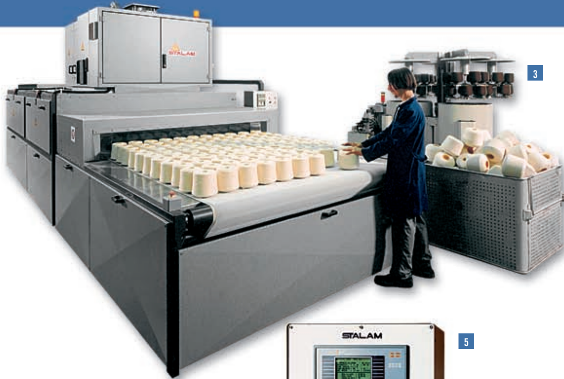
fig. 3 - “RFA 60 kW” dryer for pastel shaded wool yarn packages, hydroextracted and loaded manually.
