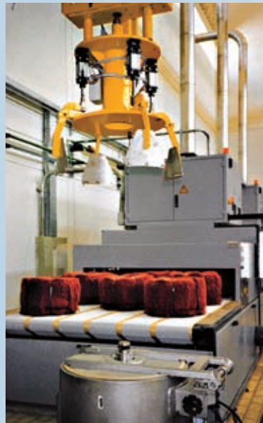
8 fig. 8 - Detail of the automation for loading and unloading tops.
