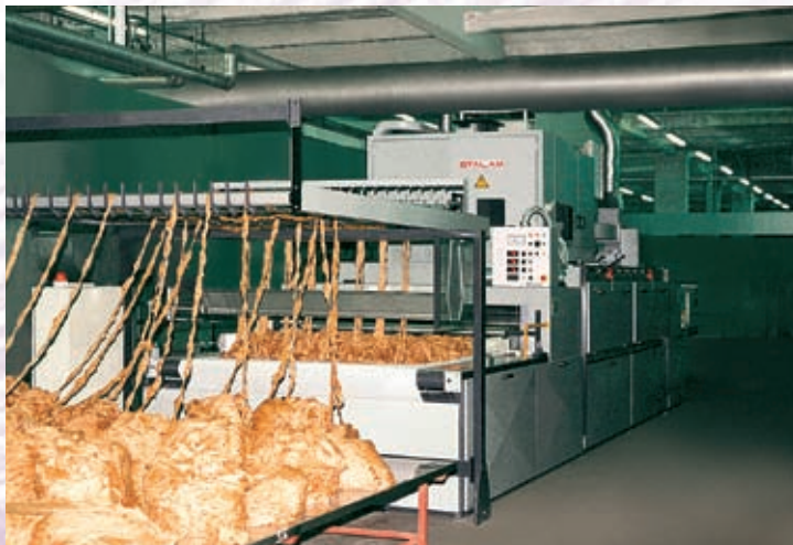
fig. 20 - “RFA/S 2x50 kW” dryer for wool and acrylic top slivers, dyed and hydroextracted in “big forms”. Slivers, at the outlet, are fed directly to the gill-box.
