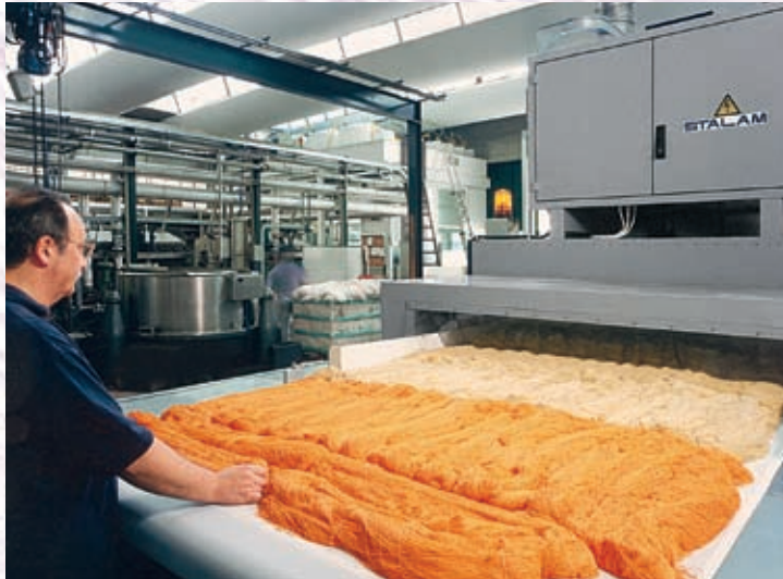
fig. 18 - “LTRF 2x60 kW” dryer for cotton and rayon knitting yarns in hank form.
