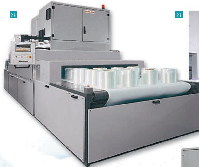
fig. 29 - "RF 75 kW" dryer for natural latex pillows and mattresses after foaming, vulcanisation, washing and roller-squeezing.
