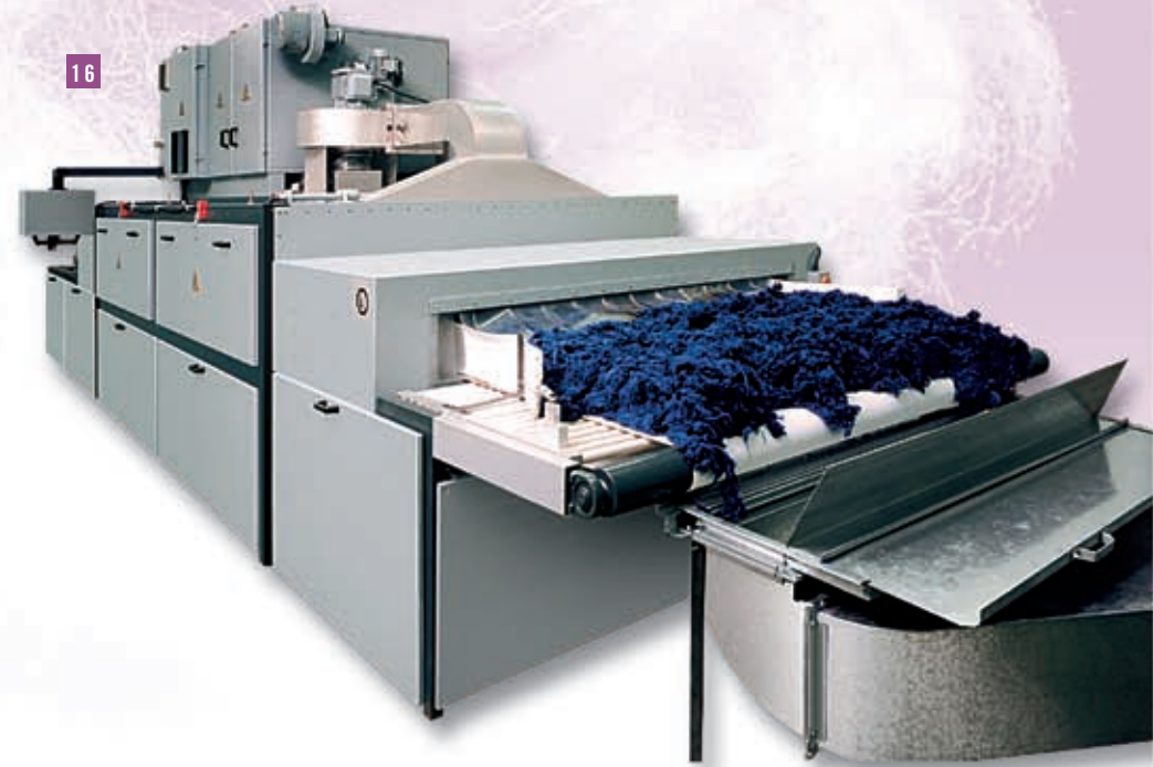
fig. 16 & 17 - "LTRF 60 kW" dryer for cotton loose stock for "mélange", with volumetric hopper feeder and unloading with pneumatic transport to storage.
