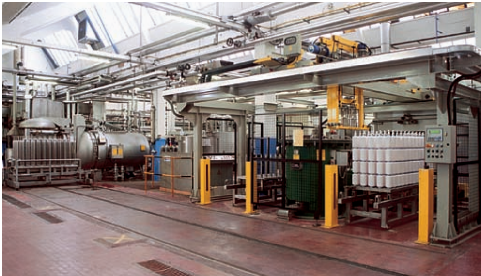
fig. 14 & 15 - “TCRF 2C/R” dryer for filament rayon yarn packages, integrated into a fully robotised dye-house.
