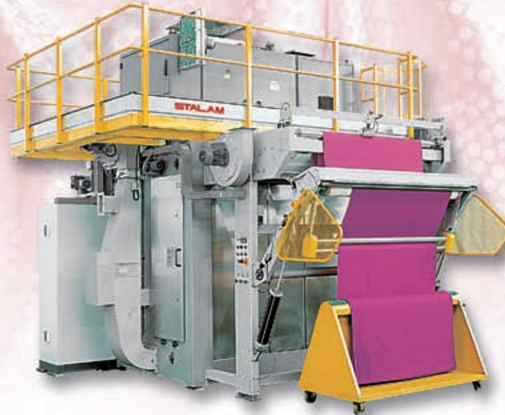
fig. 21 & 22 - “RF/T 60 kW” dryers for the drying and conditioning of high-quality woollen fabrics.
