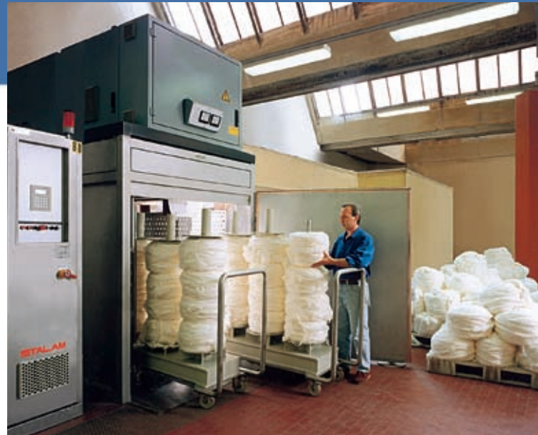
fig. 13 - “TCRF 2C/RT” dryer for fine wool tops for underwear, both in bump and bobbin form, after bleaching and anti-shrinking treatment.
