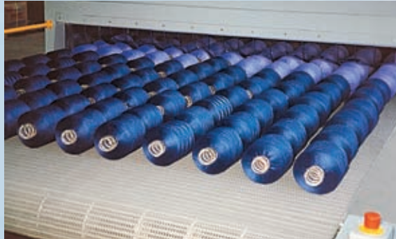
6 fig. 6 - Drying of yarn packages wound on stainless steel springs.
