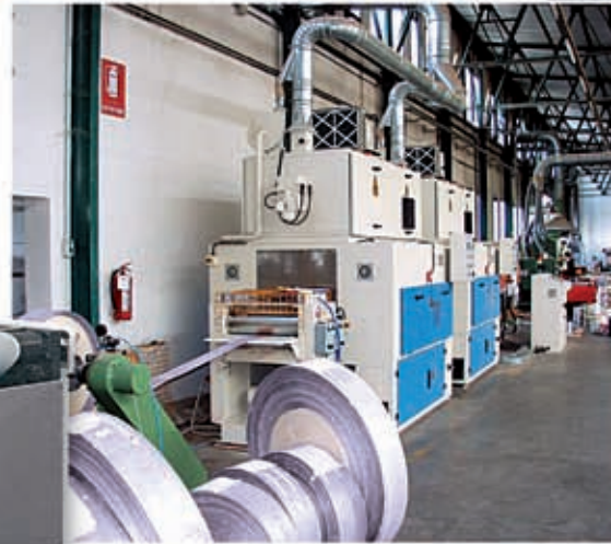
fig. 26 - "RF 60 kW" dryer for "direct roving" glass-fibres.
