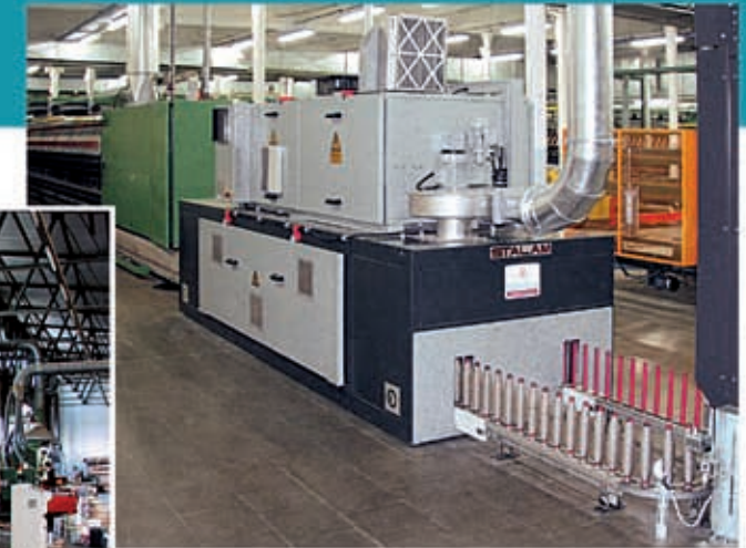
fig. 26 - "RF 60 kW" dryer for "direct roving" glass-fibres.
