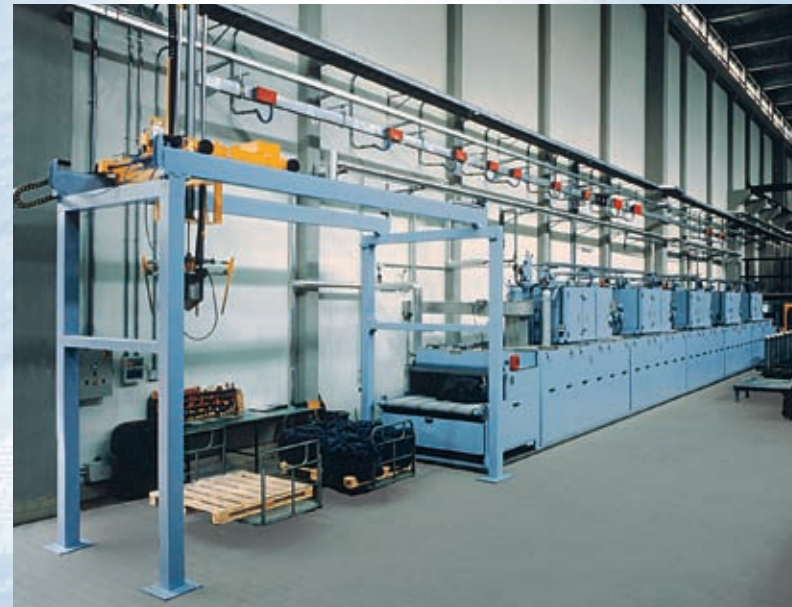
9 fig. 9 - "RF 5x40 kW" dryer for the drying of 16 ton/day of fine wool tops, 25 Kg each, hydroextracted one by one, with automated loading and unloading operations.
